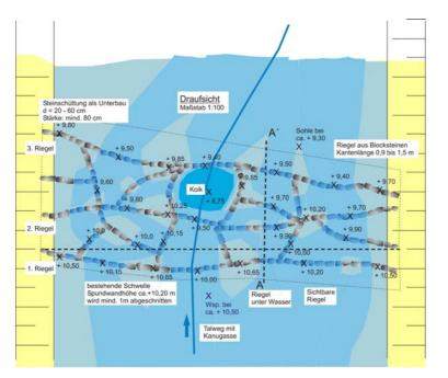
Fig. 5: Rear-defense river bank protection (schematic)
