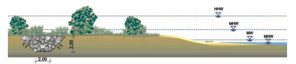
The dynamically developing banks are a special feature and are constantly changing and retreating during high water levels and flood runoff. To arrest erosion rear-defense protection measures were implemented in the forelands for safety reasons. These developing banks were provided mostly in the pilot stretch of the Isar Plan, to the south of the Marienklausensteg footbridge, where the foreland, upstream of the dyke, offers sufficient space for a controlled river development (Fig. 5).
